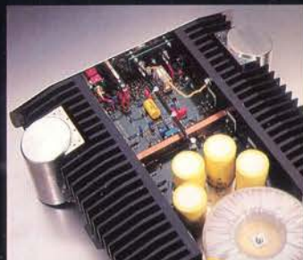
Massive, custom-designed heatsinks inside the 202 monoblock power amplifier. Note the ultra-short signal path, a benefit of the compact layout.
