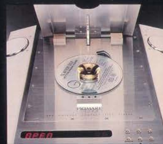
204 CD transport mechanism, with the gold-plated disc stabilizer in position.
