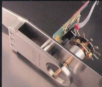
201 input selector switching via a custom-designed, non-stop pulse wheel.
